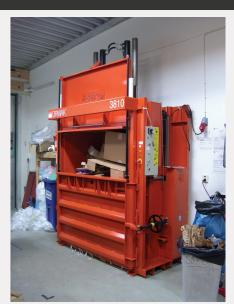
Sharp Center chose the baler Orwak 3810 for its generous loading aperture, as boxes up to 1500 mm fit easily in the infeed. The baler is placed directly at the source of waste, where boxes are received. Emil adds:
