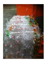
The four straps keep a firm grip on the PET-bale. The bales from the water bottling company weigh 250 kg on average.
